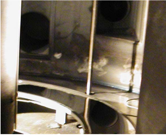
Fig. 2. Liquid lithium in toroidal tray limiter. Note the reflection on the surface of the vertical tube containing magnetic sensors near the center of the photograph.
